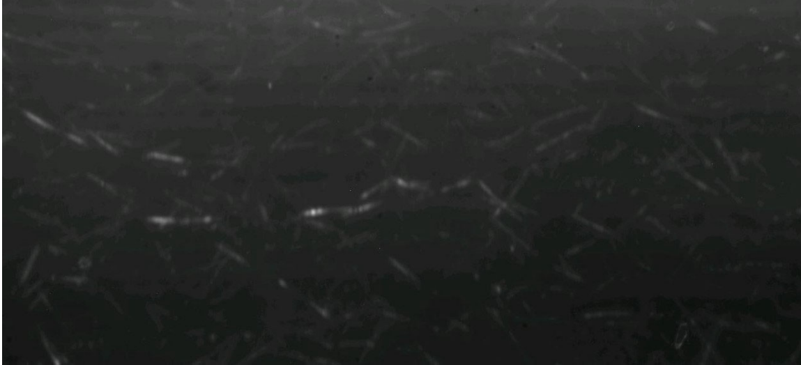
FIG. 1. USAXS image taken at q = 0.0005 \text{ \AA}^{-1} of PMMA/CB with 0.8% loading. The field of view is 0.57-mm wide \times 0.28-mm high.
