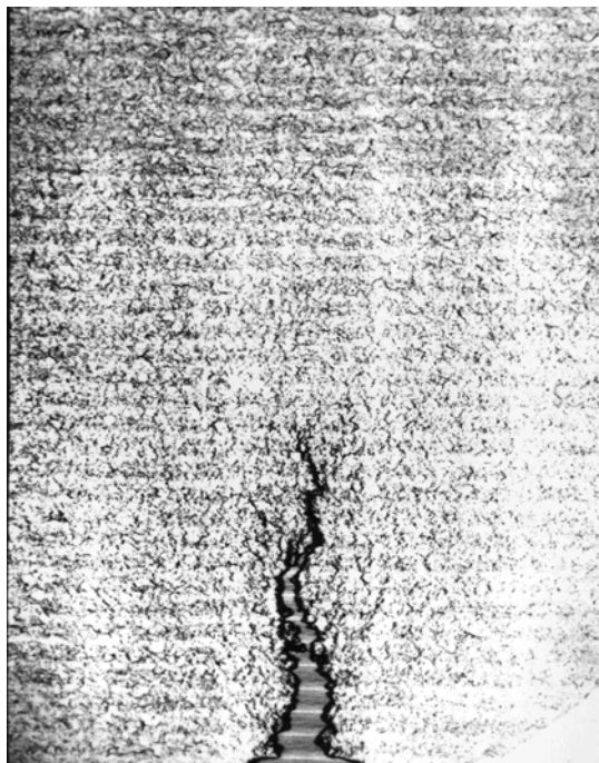
FIG. 1. Image of a crack in copper metal, taken at q = 0.0005 \text{ \AA}^{-1} with 0.9\text{-}\mu\text{m} resolution. The incident photon energy was 8.94 \text{ keV} . The microstructures near and far from the crack are the same in quality but differ greatly in quantity.
