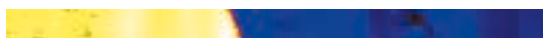
FIG. 1. Strip (1 mm × 10 mm wide) across contact between aragonite (left) and calcite (right) layers in natural high-U flowstone deposit from a cave in Austria showing U concentration image scaled in concentration from 80 ppm (black) to 500 ppm (white). Note mm-scale fluctuation in U concentration within aragonite parallel to contact. Contact was subhorizontal in field.
