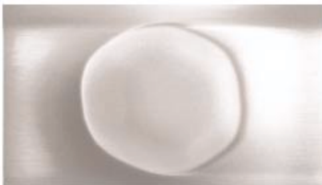
FIG. 2. Reconstructed image of one of the gold nanocrystals (left) and a scanning electron microscope image from the same preparation, displayed on the same scale for comparison (right).
