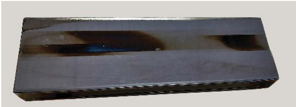
*Damaged multilayer optic before the refurbishment process
